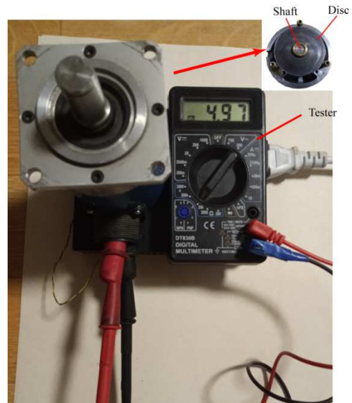
Figure 4. Experimental Setup to measure a relationship between brightness of image and output resistance of LDR.
